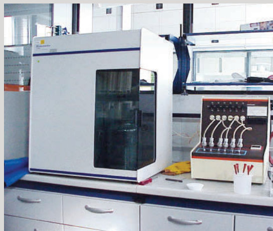
2) Measurement of nitrogen surface area/STSA
